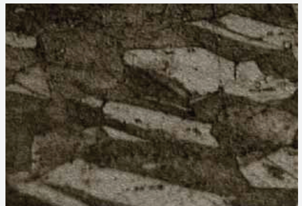
Conventional CuCrZr grain structure
