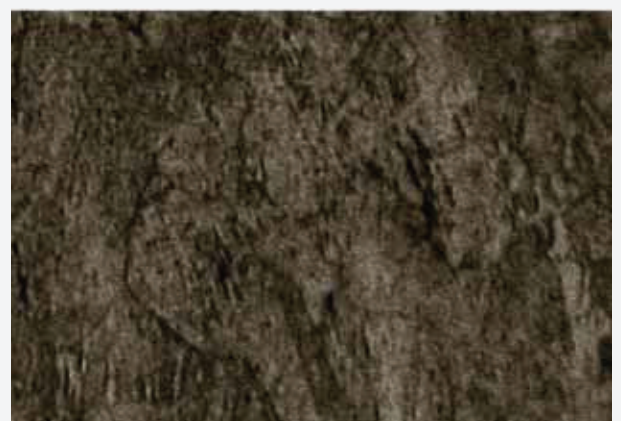
Luvata CuCrZr fine grain structure
